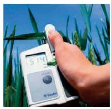
1.Simplicity and flexibility of use: The measurement is done by pinching the leaf, on or off the field. The N-Tester® is used from stage 2 leafs to swelling. In addition, you can make your measurements whatever the time of the day..
