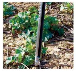
PRO-Sonde® comes with a chisel head which facilitates the pushing process by reducing friction. In addition, the small diameter allows for an easy penetration.
