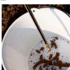
The well-sized collection channel samples the right amount of soil. Between 300 and 500 g in just 10 samplings. Sub-sampling is therefore avoided.
